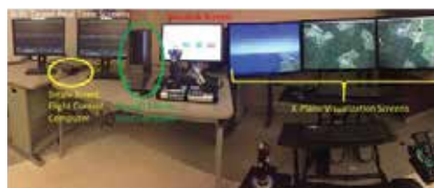
Hardware-in-the-loop (HIL) approach applied to support pilot training and autopilot development in the Flight Dynamics and Controls Laboratory
