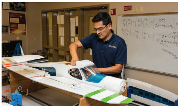
UAV testbed to support research and development of fault tolerance flight control systems.
