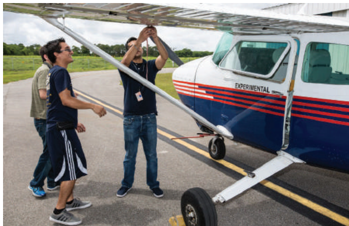
Cessna 182 adapted into a Surrogate UAS to support research and testing.
