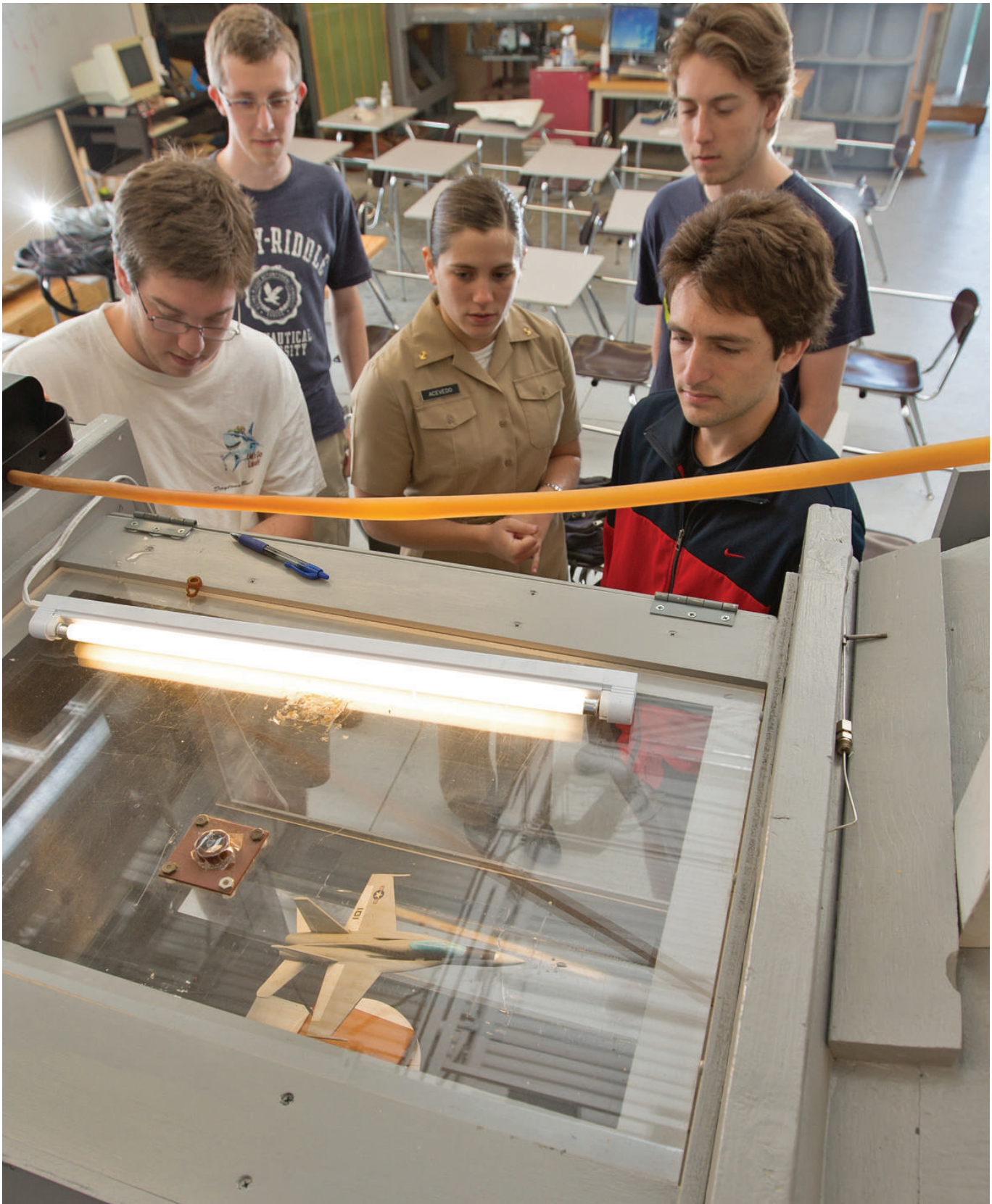
Students test various objects in the wind tunnel and record the results using iPhone video for later analysis.
