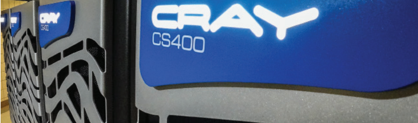
Figure 1: Vega; ERAU's four-cabinet Cray CS400™, with 3,024 cores and estimated performance of 3 Tera FLOPS.
