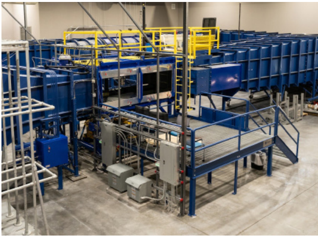
Figure 2: The test section of the wind tunnel is comprised of more than 65% optical grade glass, and is reached from elevated work platforms on two sides. The windows on both sides can be opened giving unimpeded access.
