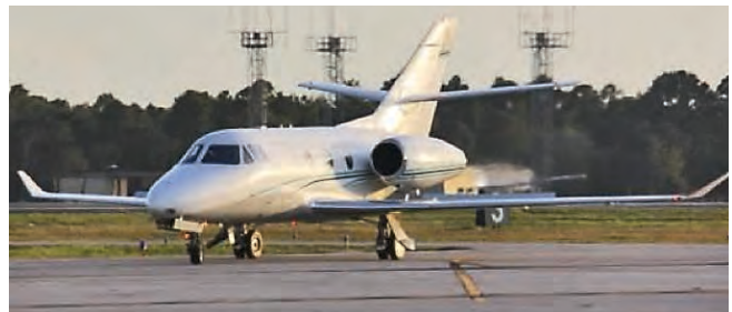
A Falcon 10 with the winglets designed by the ERAU students
